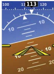
Figure 2-8 Sky Pointer Configuration
