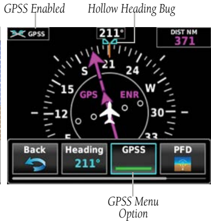
Figure 4-4 GPSS Enabled (HSI Page)
