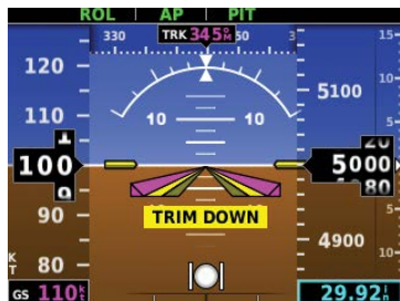
Figure 3-22 TRIM DOWN Alert
