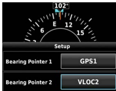
Figure 2-19 Bearing Pointer Setting
