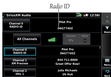
Accessing the SiriusXM Radio ID (Channel 0)
