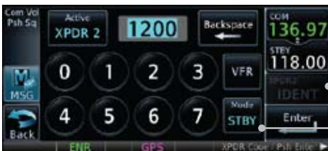
Figure 2-7 Transponder Mode "Standby" Indication
