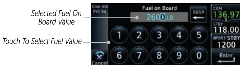
Figure 14-30 Selecting Current Fuel On Board
