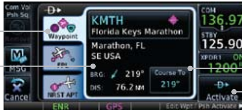
Figure 5-5 Selected Direct-To Flight Plan Leg
