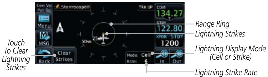
Figure 11-42 StormScope Display (360° Display View Shown)
