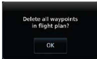
Figure 4-46 Delete a Flight Plan from the Active Flight Plan
