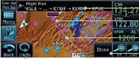
Figure 8-35 Confirm Flight Plan to New Waypoint
