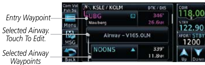
Figure 4-23 Airway Waypoints in the Flight Plan
