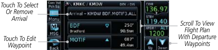
Figure 6-14 Flight Plan With Arrival Loaded
