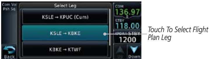
Figure 14-35 Select Flight Plan Leg
