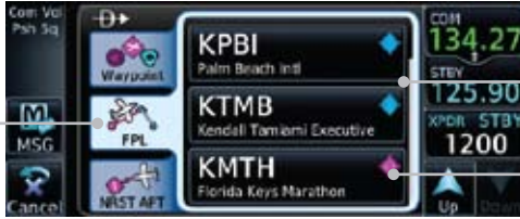
Figure 5-4 Direct-To Flight Plan Leg Selection
