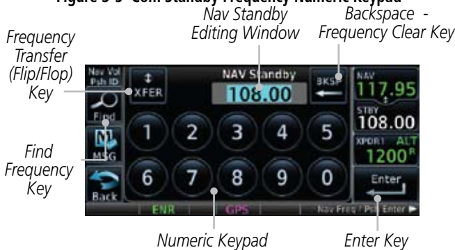
Figure 3-6 Nav Standby Frequency Numeric Keypad
