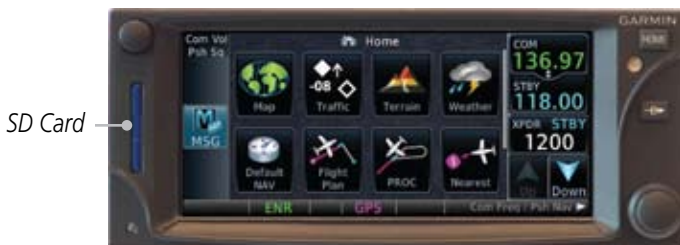
Figure 18-1 SD Card Database Location
