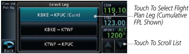
Figure 14-24 Select Flight Plan Leg
