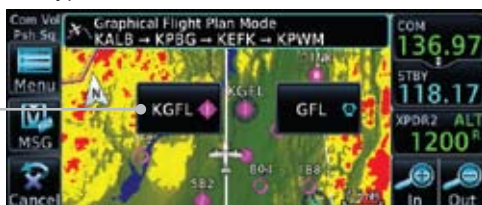
Figure 8-37 Select the Desired Waypoint From Multiple Waypoints
