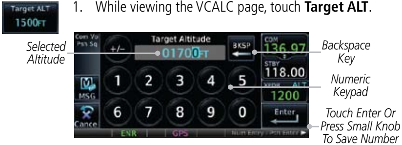
Figure 14-6 Select VCALC Target Altitude
