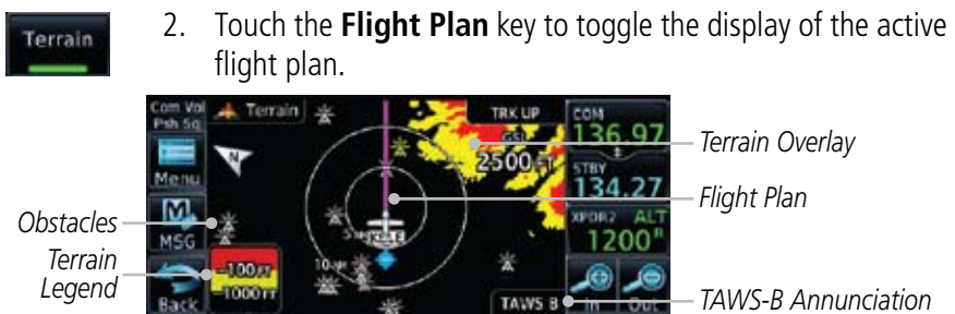
Figure 10-8 Flight Plan and Legend Shown On Terrain Page
