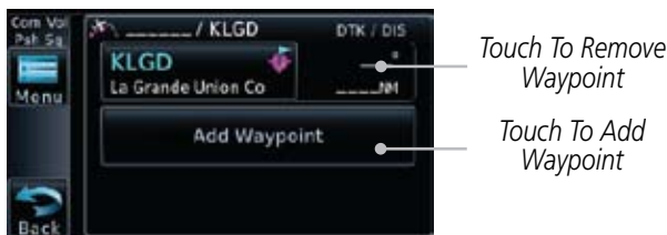
Figure 4-2 Create New Flight Plan
