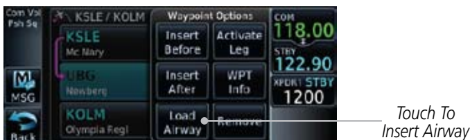
Figure 4-18 Select Load Airway from the Waypoint Options
