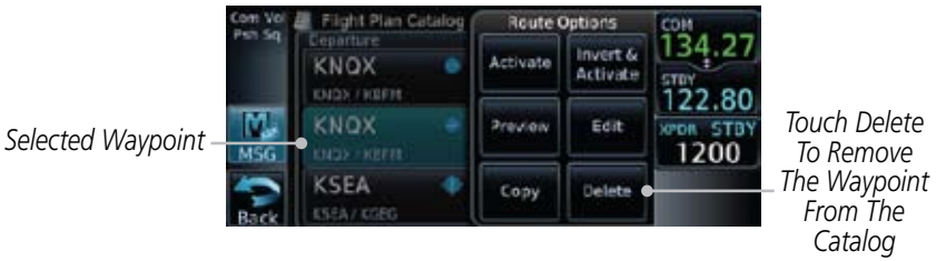
Figure 4-44 Select a Flight Plan from the Catalog
