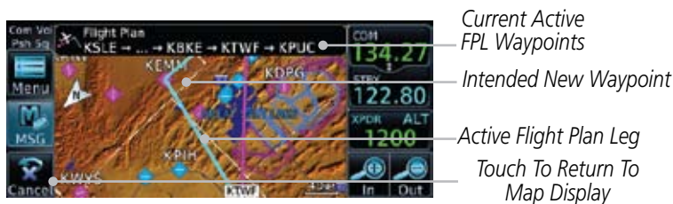
Figure 8-34 Drag Selected Leg of Flight Plan to New Waypoint
