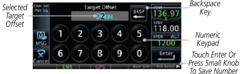
Figure 14-8 Select VCALC Target Offset
