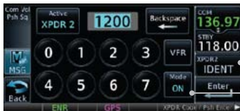
Figure 2-9 Transponder Mode "ON" Indication
