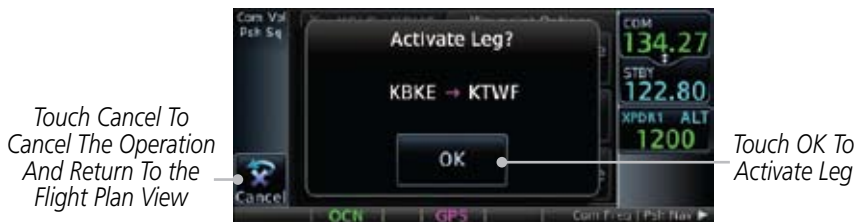
Figure 4-10 Active Flight Plan Activate Leg Option
