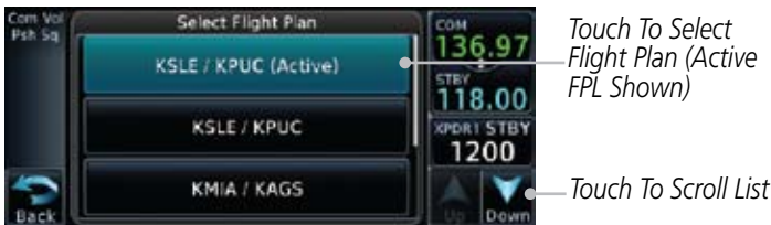
Figure 14-34 Select Flight Plan
