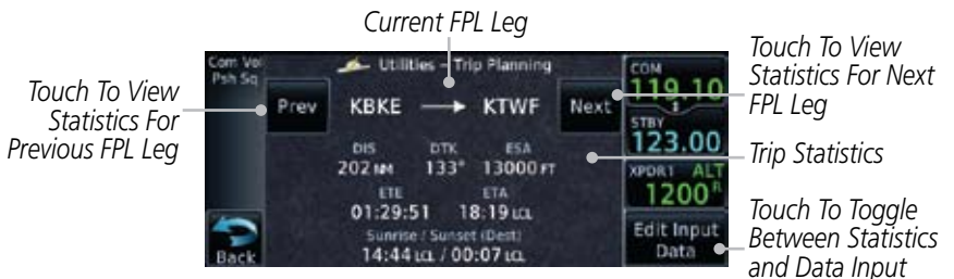
14-26 Utility Trip Planning Page Computed Data View Of Next Waypoint (Flight Plan Mode)
