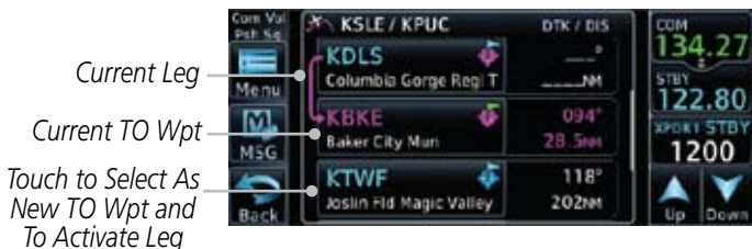
Figure 4-9 Active Flight Plan Activate Leg Option
