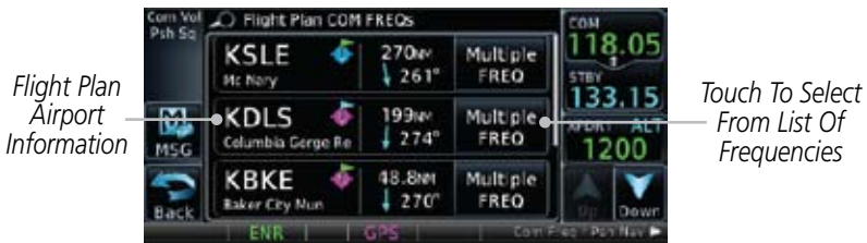
Figure 3-14 Flight Plan Frequency List
