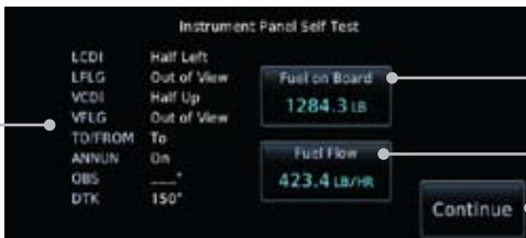
Figure 1-11 Instrument Panel Self-Test & Fuel Settings Page
