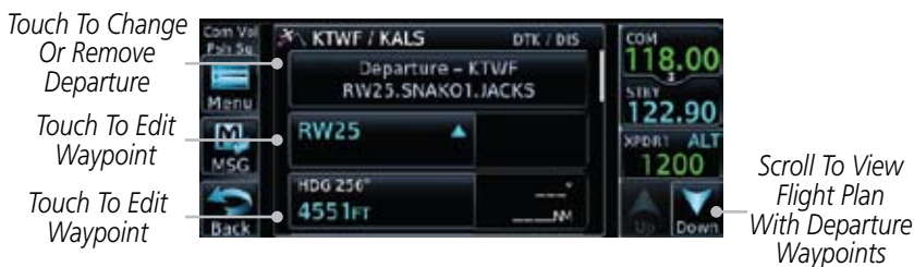
Figure 6-7 Flight Plan View of the Selected Departure
