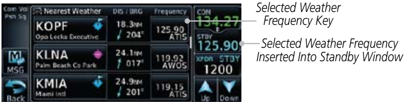
Figure 12-23 Nearest Weather Station Selected Frequency
