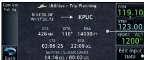
Figure 14-21 Utility Trip Planning Page With Computed Data (Point-To-Point Mode)
