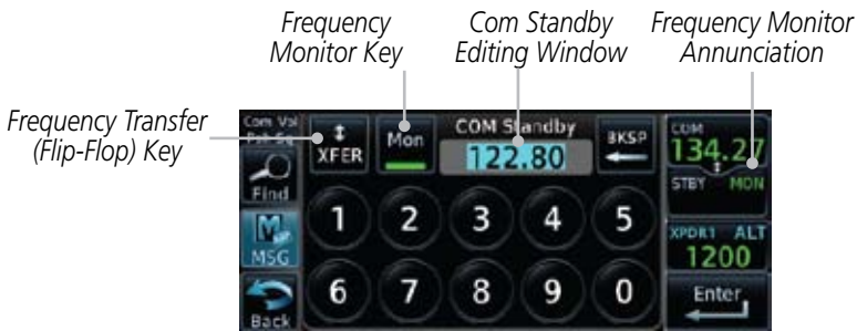
Figure 3-21 Com Frequency Monitoring
