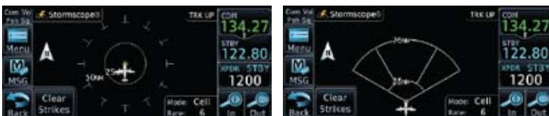
Figure 11-44 StormScope 360° and Arc Display Views
