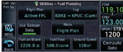
Figure 14-33 Utility Fuel Planning Page Showing Edit Input Data (Flight Plan Mode)
