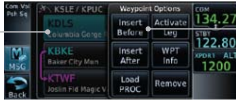
Figure 4-11 Active Flight Plan Insert Waypoint Before Option
