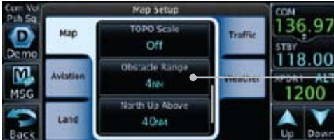
Figure 8-19 Map Setup For Obstacle Range
