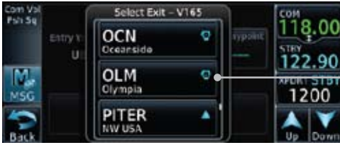
Figure 4-20 Select an Exit Waypoint for the Airway
