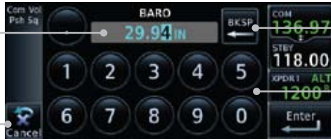
Figure 14-40 Select Barometric Pressure Value
