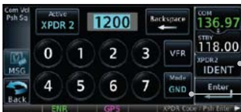
Figure 2-8 Transponder Mode "Ground" Indication
