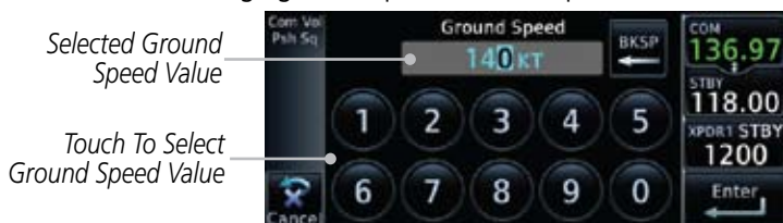
Figure 14-32 Selecting Ground Speed
