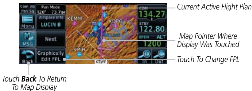
Figure 8-33 Edit Flight Plan Mode
