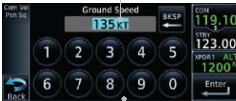
Figure 14-20 Selecting Expected Average Ground Speed
