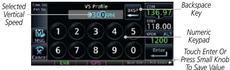
Figure 14-7 Select VCALC Vertical Speed
