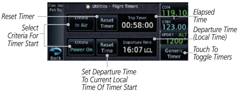
Figure 14-12 Utility Flight Timers Page (Trip/DEP Timers)
